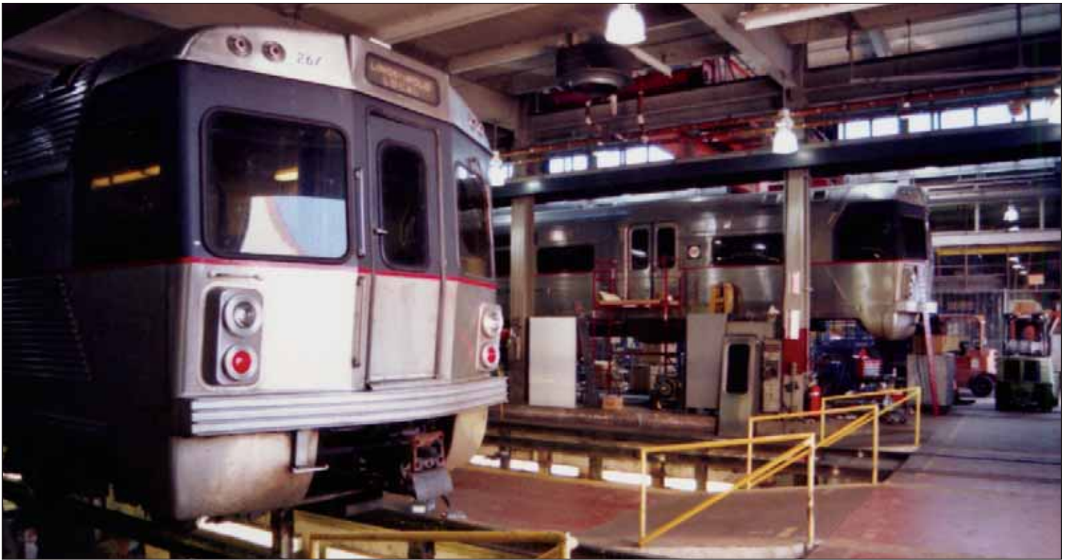
2/13/04 7:27PM Trains are serviced around the clock at PATCO's Lindenwold Shop. PATCO train cars log on average 35,000 miles a year.
