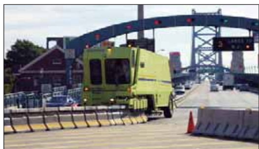
5/3/04 1:35PM Twice a day, workers adjust the Ben Franklin Bridge's moveable barrier to favor peak-direction travel. The Walt Whitman and Commodore Barry bridges also have moveable barriers.
