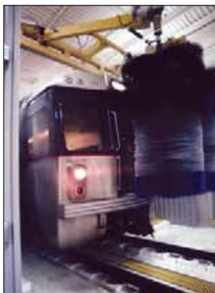
11/01/04 2:32PM DRPA began initial test runs of the new PATCO car wash in late 2004. The new car wash can clean the cars without any supervision.
